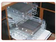
According to owners guide, recommended maintenance involves frequent vacuuming, washing, and a technical service call to wipe the sharp tips of the field-charger. Filter performance decreases 5% after first vacuuming.
